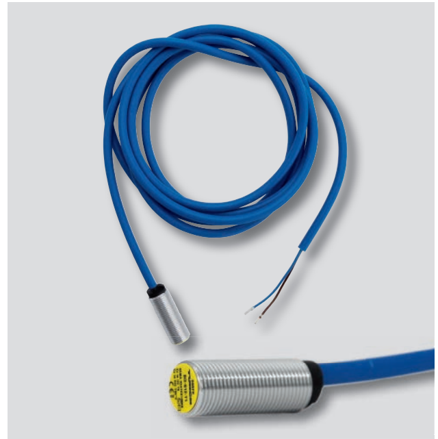
Rotational speed sensor with 2 wires, Namur.
