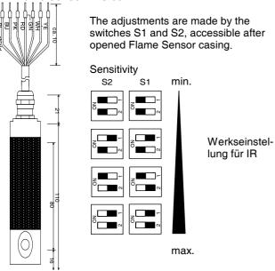
The min. threshold value for IR-Flame Sensors are 15 mV and for UV-Flame Sensors 25 mV. Further information for operation of the Flame Sensors are given in the technical documentation for the Flame Detector Devices.
